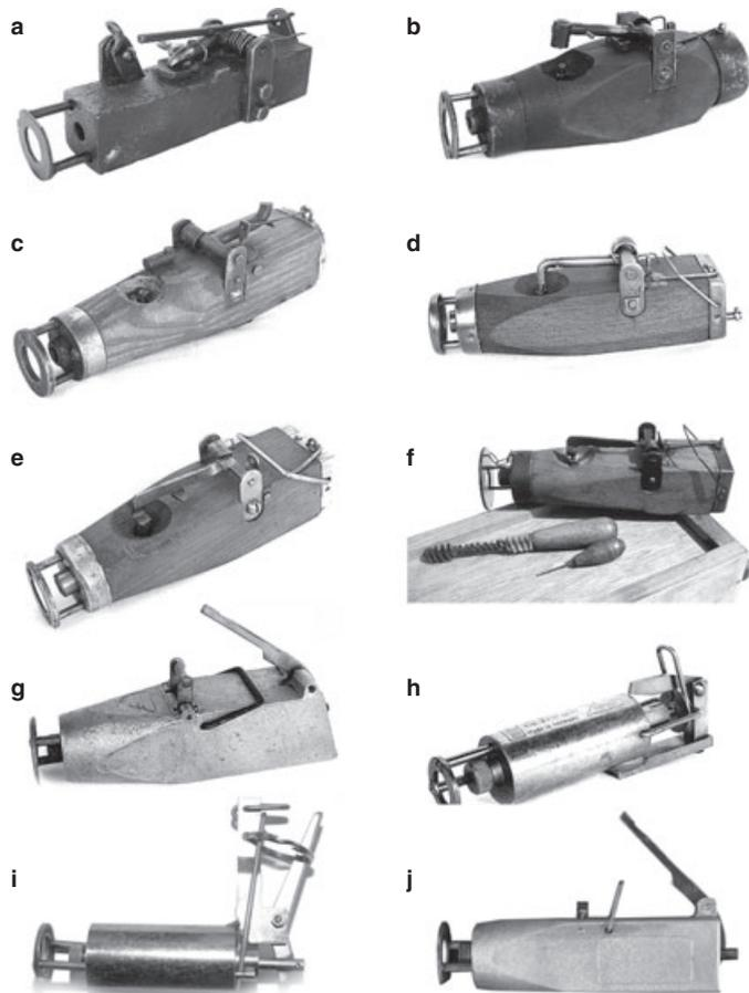
FIG. 3—Technical development of powder actuated vole captive bolt devices. Muzzle-loading blackpowder shooting traps were developed in the Lake Constance area from the 1930s (a–f). In the 1950s they were technically refined and featured a screwable cartridge chamber. Since then, they have been mass-produced (g, h). Today, two different models are approved and commercially available (i Model Kieferle W2, j Model Auber Aura).
