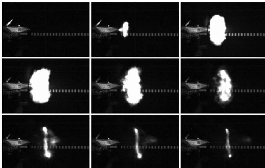
FIG. 2—High-speed motion analysis of the muzzle flash of a vole captive bolt device (High-speed camera MotionXtra HG-100K, Redlake Digital Imaging Systems, Tallahassee, USA; frame rate 5000 frames/s). The initial muzzle flash consists of a fire-jet that streams out of the muzzle. The second flash is due to combustion of unburned gases ( $H_2$  and  $CO$ ) that leave the muzzle and react with the oxygen of the air surrounding the muzzle.
