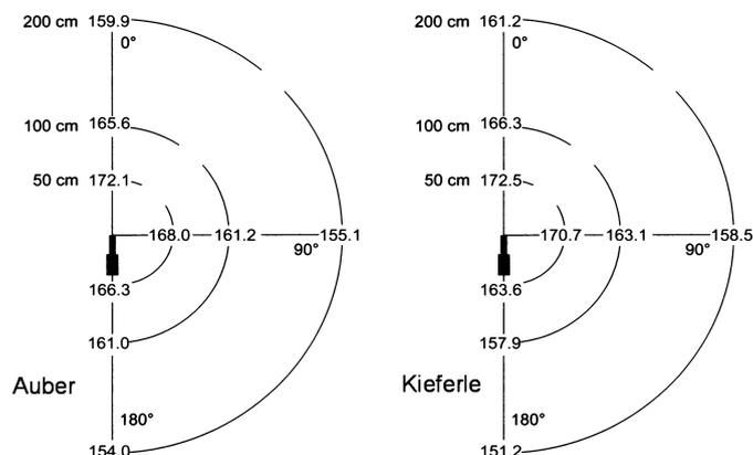
FIG. 6—Geometric distribution (near field) of the sound pressure levels (SPL in dB[C]), average value of 10 shots at each location (left: model Auber Aura, right: model Kieferle W2). Style of graphical data presentation with reference to (12).
