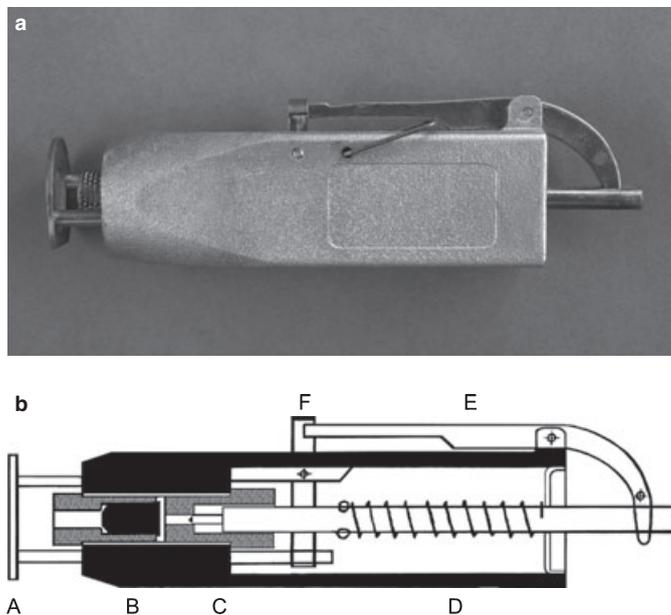
FIG. 1—(a) Vole captive bolt device (Model Auber, approval number PTB 2). (b) Functional principle. The shooting trap is loaded with an industrial blank cartridge through the screwable explosion chamber B. Trigger mechanism A, firing pin C, firing pin spring D, cocking lever E, trigger device F.
